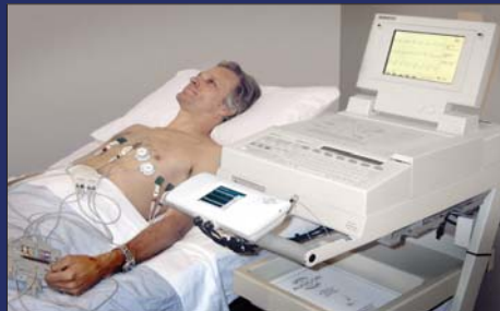
Figure 1 The Audicor add-on device (white) attached to an existing ECG.
